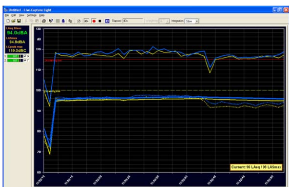
Sound level logging according to IEC 61672 standard. Graph shows LAFmax, LCpeak and LAeq.
